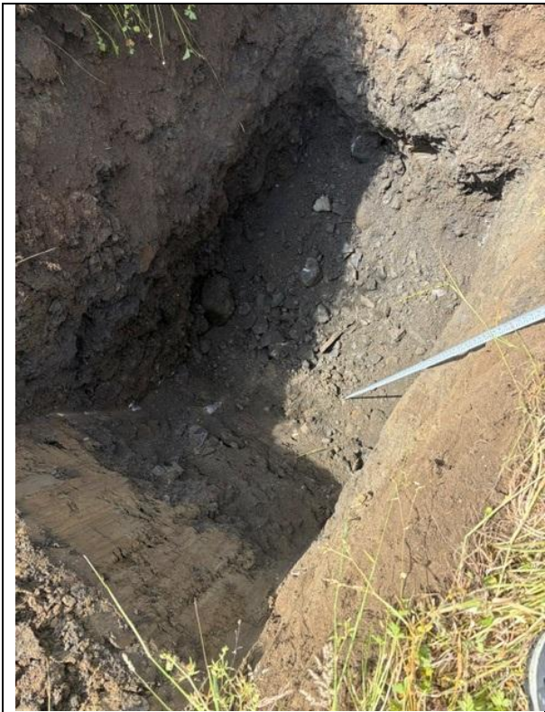
Trial Hole 3 – Dug to 2.1m Gravel with rounded and angular boulders
