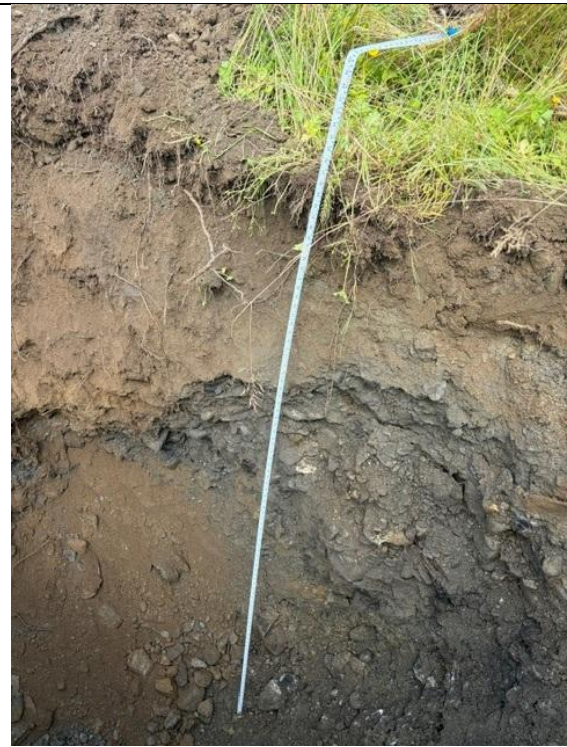
Trial Hole 4 – Dug to 2.2m Gravel with rounded and angular cobbles/stone.
