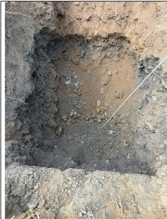
Trial Hole 4 – Dug to 2.2m Gravel with rounded and angular cobbles/stone.
